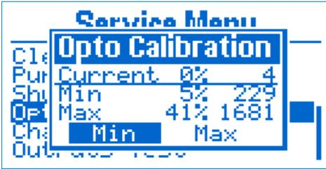
Fig 16 Flame sensor calibration
