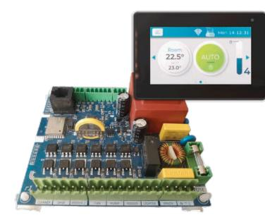
The product design is focused on the easy and convenient setup, ensuring the smooth installation process of the heating system. Furthermore, internet monitoring and event logging makes the tuning of system performance easy.
